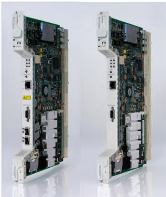
Figure 1. Cisco ONS 15454 TNC Card and ONS 15454 TSC Card
